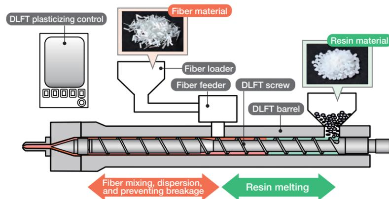
A fusion of the specially developed DLFT screw using an inline screw method together with our plasticizing control technology
